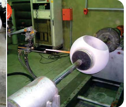
STELLITE OVERLAY THROUGH HVOF PROCESS
