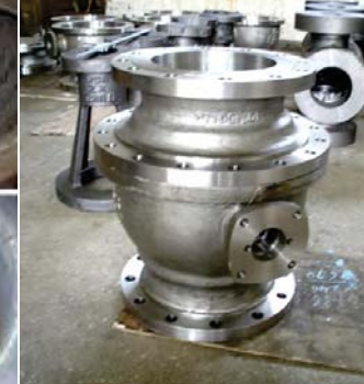
STELLITE OVERLAY AFTER MACHINING
