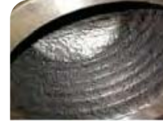
STELLITE OVERLAY BEFORE MACHINING
